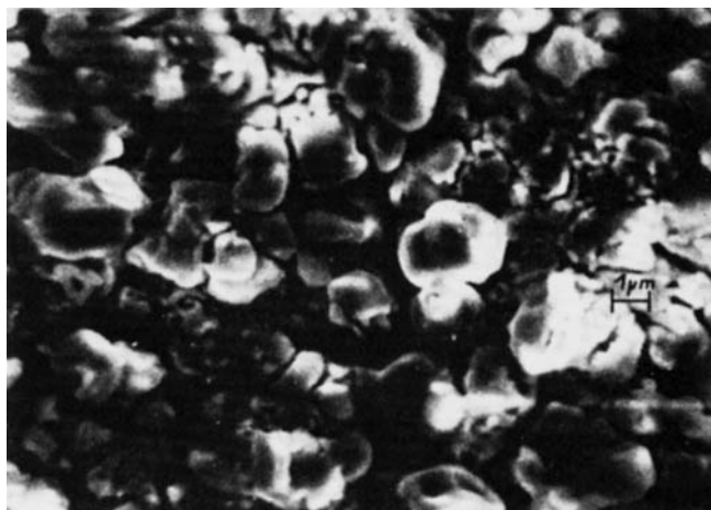
Figure 7. Enlarged view of surface of oxide-ceramic covered metal screen.
